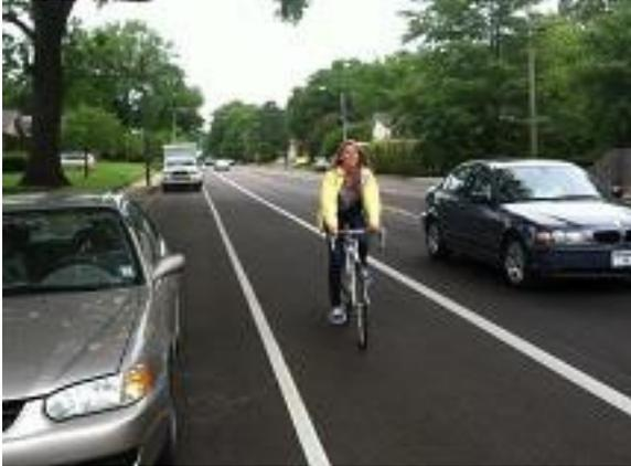
**Marked bike boulevards:** Also known as neighborhood greenways are streets with low motorized traffic volumes and speeds that have been designated and modified to function as a through street for bicyclists using signs, pavement markings, and traffic calming measures to discourage through travel for motor vehicles.
